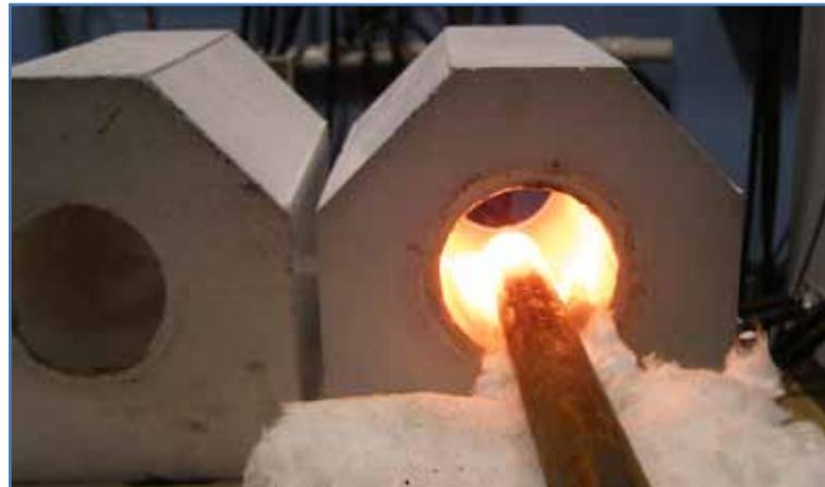
*Heating a 75 mm diameter bar to 1100°C (2012°F) for hot heading. An eight-position coil was used to provide one hot bar end every 20 seconds to the robot for loading into the press.*
